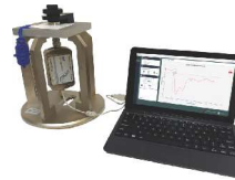
Epsilon meter Freq. Range : 3MHz~6GHz Impedance : 50Ω Sheet thickness: 0.3~3mm Suitable for Ceramics testing
